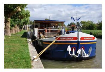
Former purpose: Ex French cargo carrier Year of construction: 1960 128ft (39m) x 17ft 6" (5.3m) **Dimensions:** Year converted into a hotel barge: 1997 Cabins completely refurbished: 2015 Generators: 2 x 220 volt generators Main engine 250 HP BAUDOIN Main engine: Maximum speed: 10 knots Water & fuel capacity: 6 tons of water & 3 tons of fuel
