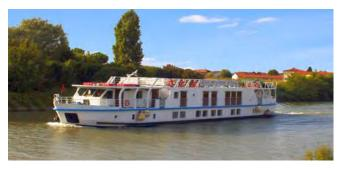
Former purpose: Sand barge on the River Po Year of construction: 1960 21.6ft x 147.6ft (6.6m X 45m) Dimensions: Year converted into a floating hotel: 2010 Generators: Main engine: AIFO IVECO SRM55M (550 Horse Power x 2) Maximum speed: 10 knots Water capacity: 20,000 litres 12,000 litres Fuel capacity: Cruise distance: 174km
